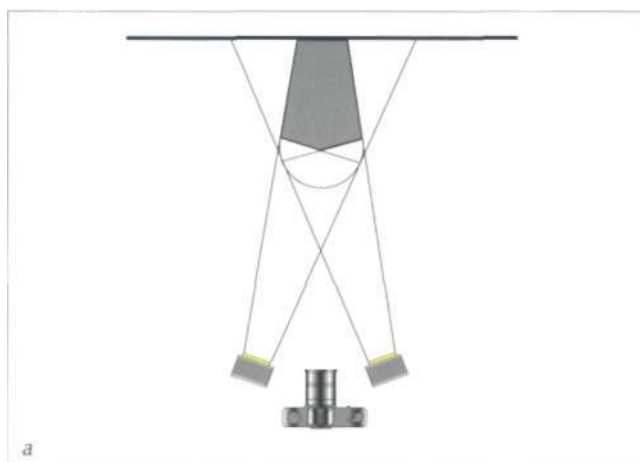
Fig. 2.46 Using a bilateral flash (a) provides high light output and even illumination. An example of such a flash bracket system is the BINZ flash, a handmade high-end system.
