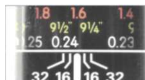
Fig. 2.20c Magnification ratio of 1:1: 36mm are visible within the frame. Corresponding magnification ratio number of a Nikon lens (orange values).
