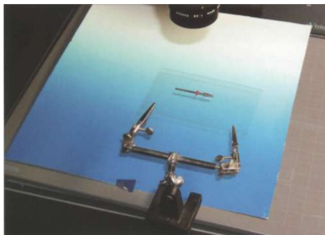
Fig. 7.12 Isolation of a small object using a simple glass plate.
