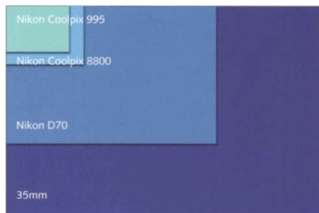
Fig. 3.6 Sensor size of different cameras in relation to 35-mm film format.
