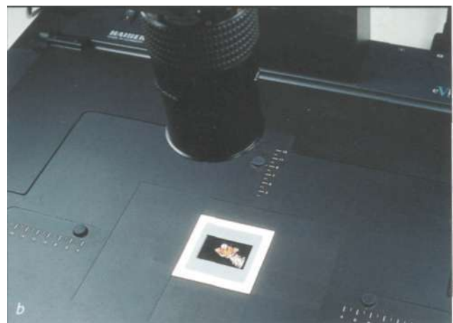
Fig. 11.3 A mask frame on a light box is also very good for copying slides (a). If the area around the slide is left free to some extent, this also reduces contrast (b).
