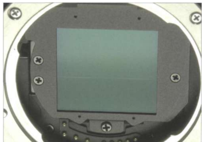
Fig. 16.24 In the Sigma SD-10, the sensor is protected by a glass filter covering the camera opening.
