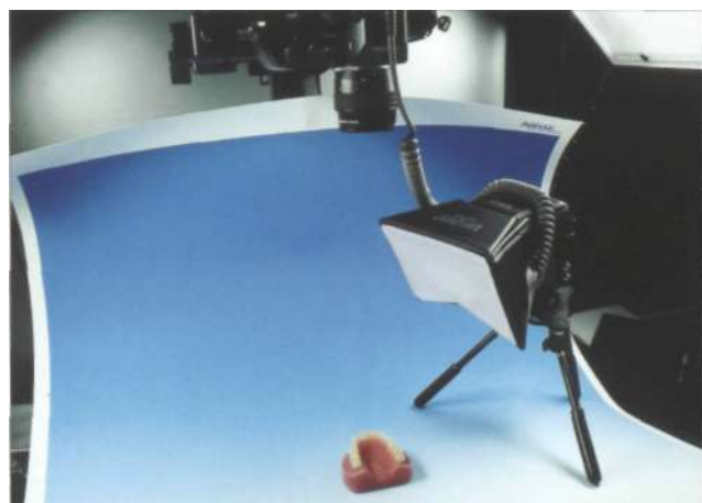
Fig. 7.34 If electronic flash is used for technical photography, the beam of light should be spread by using a diffuser.
