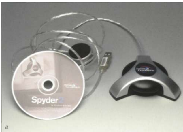
Fig. 17.08 Spyder2 device from ColorVision (a). Spyder during calibration process (b).
