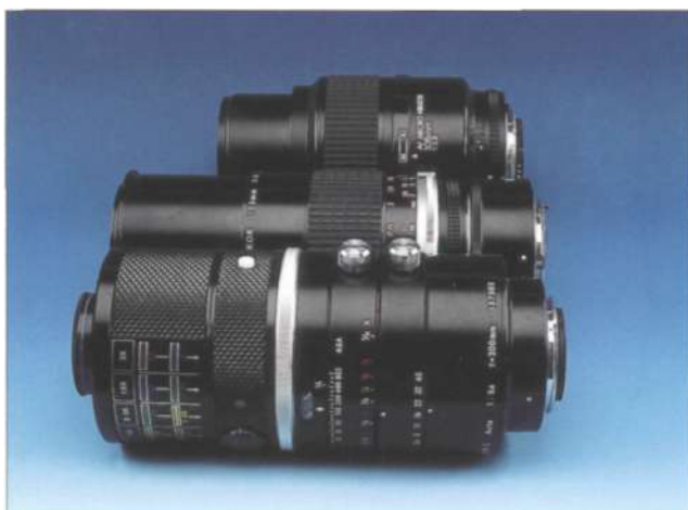
Fig. 2.10 Nikon macro lenses. In front, the old 200-mm medical lens; in the middle, a 105-mm macro lens which achieves a magnification of 1:2; in the back, the newer 105-mm AF macro lens which achieves a magnification of 1:1. Despite the greater magnification, it is physically shorter than the other lenses, since it has floating lens elements. However, this also has a shorter subject-to-camera distance.
