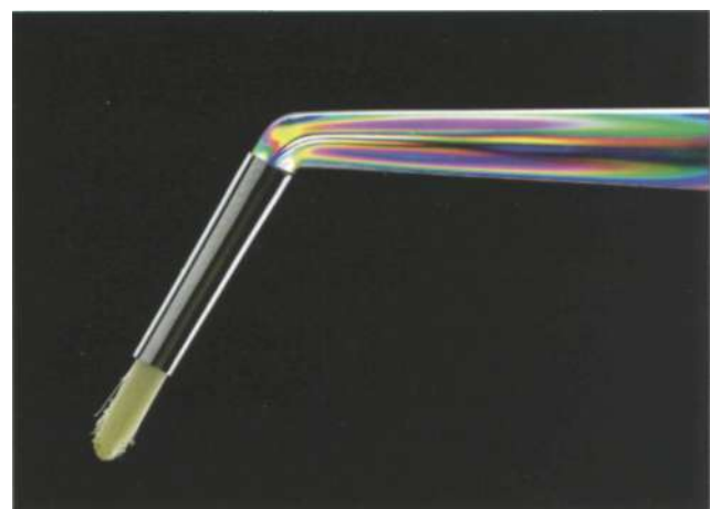
Fig. 7.70 Polarized transmitted lighting is also used for showing mechanical stresses. Internal mechanical stresses are rendered as color bands. The image shows this type of mechanical stress in the handle of a small brush.
