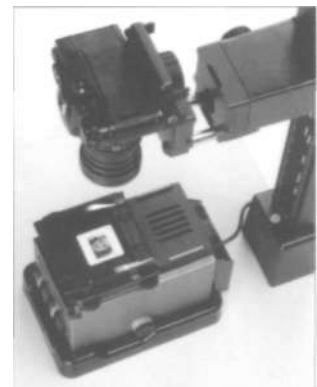
Fig. 11.4 The color head of a color enlarger is well suited to slide copying since the color of its light can be changed as desired (Photo: Kaiser).
