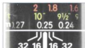
Fig. 2.20b Magnification ratio of 1:1.2: 43mm are visible within the frame. Corresponding magnification ratio number of a Nikon lens (orange values).
