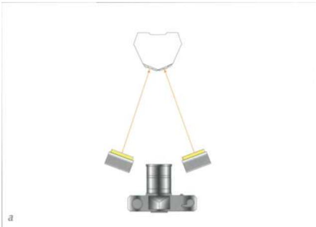
Fig. 8.9 Photograph of a cast with a twin flash system. Diagram (a) and result (b).
