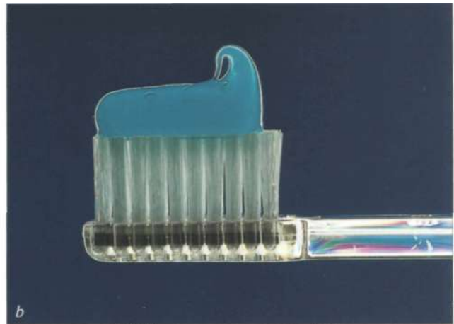
Fig. 7.67 Photographing horizontally using polarized transmitted light (a). A polarizing sheet has been fixed to a light box stood vertically. A second polarizing filter is fitted to the lens. If both polarizing filters are adjusted so that they are nearly perpendicular, the background appears dark blue (b).
