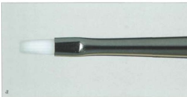
Fig. 7.67 Photographing horizontally using polarized transmitted light (a). A polarizing sheet has been fixed to a light box stood vertically. A second polarizing filter is fitted to the lens. If both polarizing filters are adjusted so that they are nearly perpendicular, the background appears dark blue (b).
