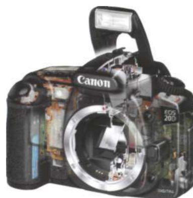
Fig 2 7 cross section of a modern digital single lens reflex camera (Illustration: Canon).
