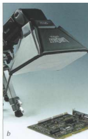
Fig. 7.43 Diagram of lighting using a diffuser and reflector, which achieves the best results in technical photography (a). The light-emitting surface of a flashgun can be increased using a soft box (b). This produces less harsh lighting (d), in contrast to the image made without using a soft box (c).
