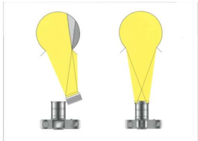
Fig. 2.43 Ring flashes are ideal for illumination of body cavities. If it is not closely enough placed to the lens, illumination by a point flash may result in shadows.
