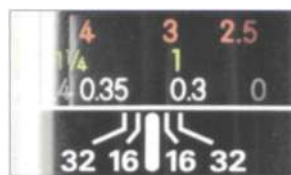
Fig. 2.20a Magnification ratio of 1:2: 72mm are visible within the frame. Corresponding magnification ratio number of a Nikon lens (orange values).
