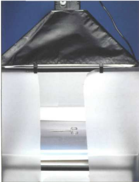
Fig. 7.35 Studio flash lights have a built-in constant light source which can be used as modelling lamp. This allows control of the distribution of light and shadow.
