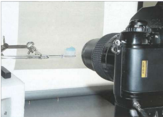
Fig. 7.67 Photographing horizontally using polarized transmitted light (a). A polarizing sheet has been fixed to a light box stood vertically. A second polarizing filter is fitted to the lens. If both polarizing filters are adjusted so that they are nearly perpendicular, the background appears dark blue (b).
