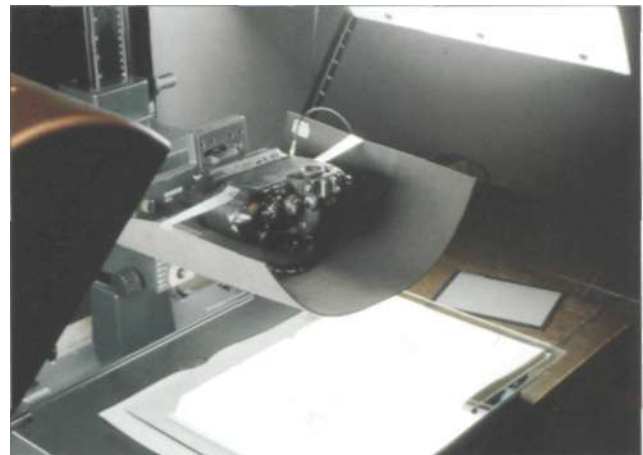
Fig. 9.7 Uneven originals can be flattened using a glass plate. The black cardboard in front of the camera prevents reflections on the surface of the glass.
