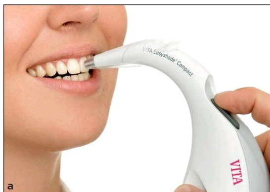
Fig 5-3 (a and b) The EasyShade compact (a spot-measurement device). The tip of the instrument is positioned on the tooth surface. Single or multiple points can be measured on natural teeth, ceramic restorations, and shade tabs. Correct positioning of the tip is crucial for correct results.
