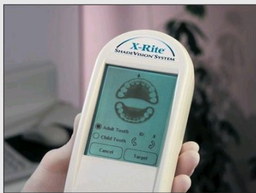
Fig 5-20a Display screen of the ShadeVision instrument on which the tooth to be measured is selected by touch.
