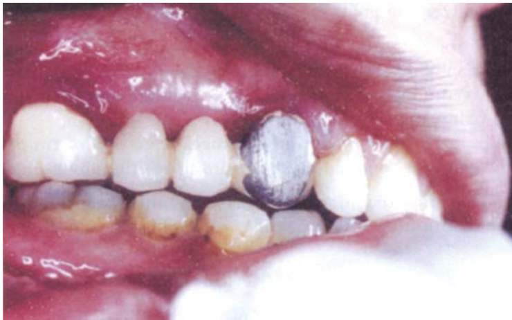
FIGURE 20.6: A failed metal ceramic bridge. The ceramic veneer (canine) has delaminated leaving the metal exposed. In this case it was because of a poorly adherent metal oxide layer
