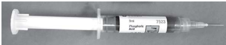
FIGURE 9.9: 37% Phosphoric acid etching agent in syringe form. The acid usually comes in a contrasting color in order to give better application control to the operator. The acid may be in liquid form or in gel form
