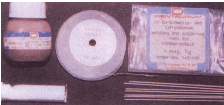
FIGURE 22.2: Representative commercial solders and fluxes
