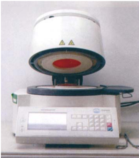
FIGURE 20.4E: After each application the porcelain is fired in a computer controlled porcelain furnace at high temperatures
