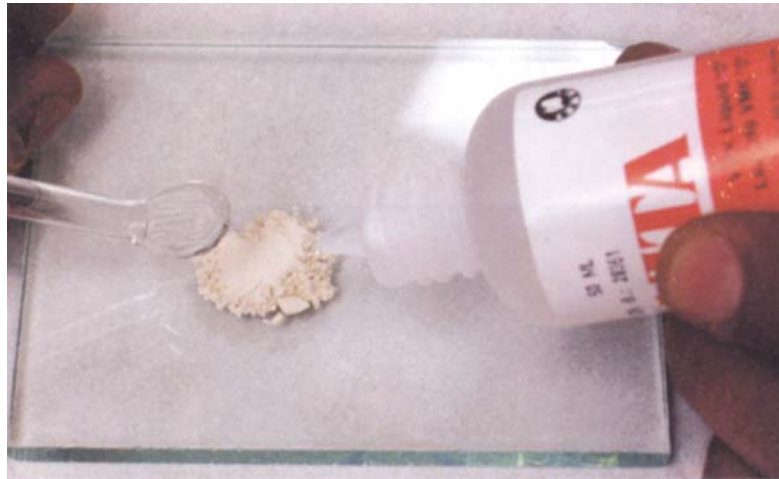
FIGURE 20.4A: Opauquer powder is a dense cream colored powder used to hide the metal. It is mixed with the modeling liquid to produce a sandy mix. A glass spatula is used for mixing as metal might abrade and contaminate the porcelain
