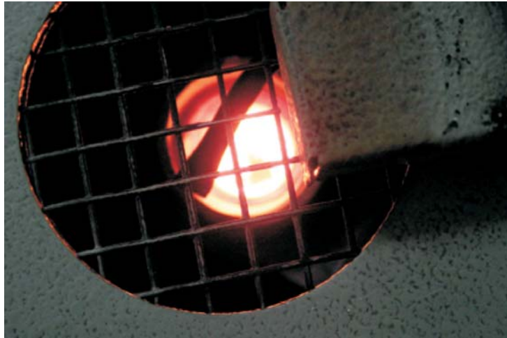
FIGURE 18.7: The above picture shows the alloy melting in the crucible. The crucible containing the alloy is surrounded by an induction coil which supplies the intense heat needed to melt the alloy pieces
