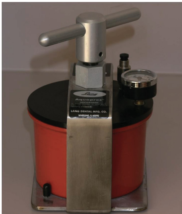
Fig. 9.15. Acrylic resin OBS cured under pressure for 10 minutes at 30 psi to reduce porosity (Aquapres, Lang Dental, Wheeling, IL).
