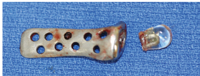
Figure 11.12 Fractured condylar head in type-I Christensen prosthesis. The type-I Christensen condylar prosthesis was made of chrome-cobalt-molybdenum alloy (Vitallium®) with a methyl-methacrylate head. It was associated with a high incidence of fracture and wear.
