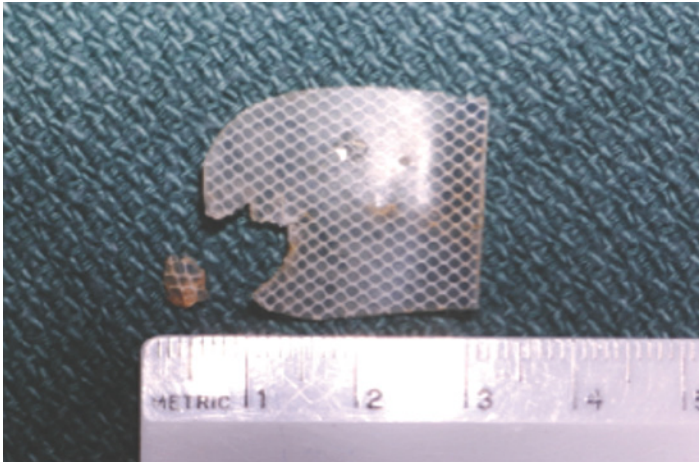
Figure 11.9 Dacron-reinforced silicone sheet showing wear and fragmentation.
