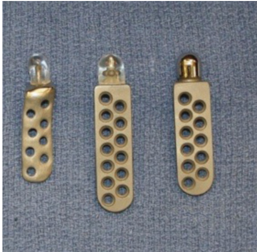
Figure 8.12 Three generation of the Christensen prostheses, from left-to-right Christensen type I, Christensen type II, and the all-metallic version. Note the methyl-methacrylate head of the type-I and type-II prosthesis.
