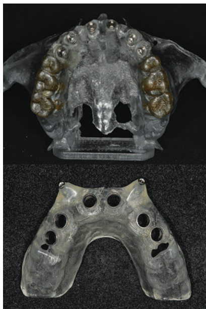
FIGURE 7.3 Stereolithographic model and surgical template were ordered. Implant analogs were set in model to allow for fabrication of abutments and interim prostheses.
