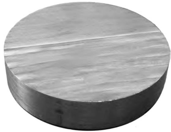
FIGURE 17.8 Titanium alloy blank prior to placement into milling machine for milling a CAD/CAM implant framework (Biomet 3i, Palm Beach Gardens, FL).
