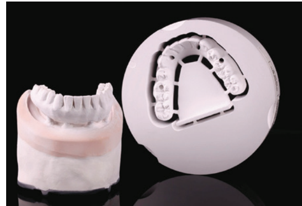
FIGURE 18.5 Milled green-state zirconia prosthesis.
