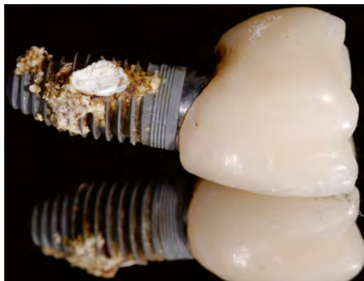
Fig. 2.10 Another failed implant with residual excess cement noted all the way down onto the screw threads. It should be stated that cement may not be the cause of failure in some cases; however, the lack of control of the clinician with the cementing technique is clear
