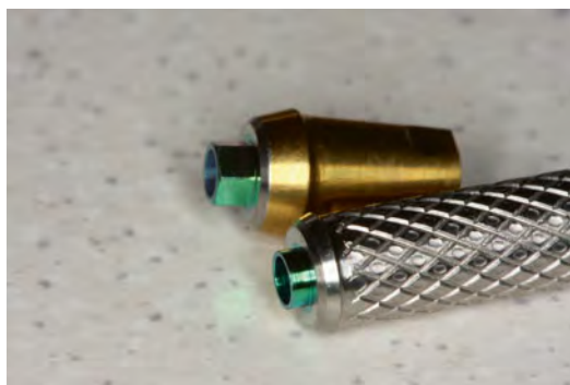
Fig. 7.26 The difference between abutment for single restorations (yellow abutment) and base for fixed partial denture. Note the absence of hex indexing, although conus connection is the same in both abutments
