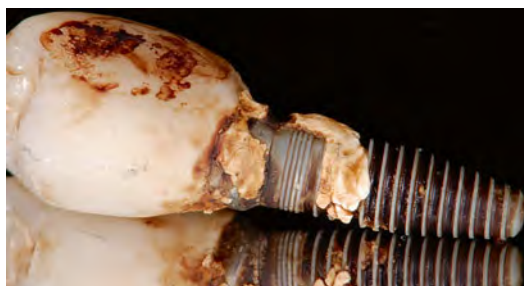
Fig. 3.31 This implant had material one-third along the body length. Evaluation by spectrometer profiling identified this had chemistry consistent with luting cement (see Chap. 2)
