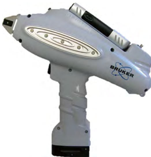
Fig. 2.14 The Bruker TRACeR III-V X-ray fluorescence analyzer (Photo courtesy of Bruker Elemental, Kennewick, WA, USA)
