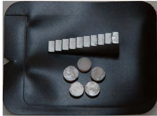
Fig. 5.4 Specimen disks with modified step wedge
