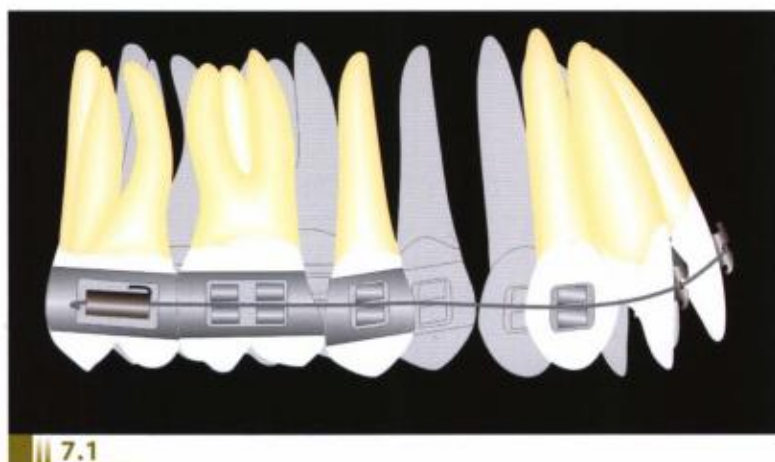
Fig. 7.1 – Newton's Third Law of Motion applied to Orthodontics. Retraction forces applied to the anterior teeth are equal and opposite to mesialization forces on posterior teeth.
