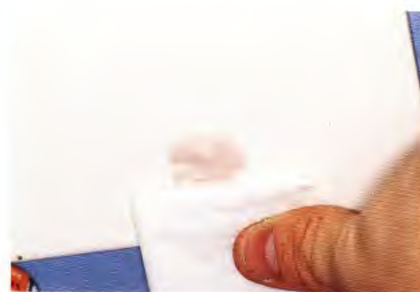
Fig 8-39 If too much liquid is added to the mix, use a tissue or blotting paper to remove excess liquid until the proper consistency is achieved.
