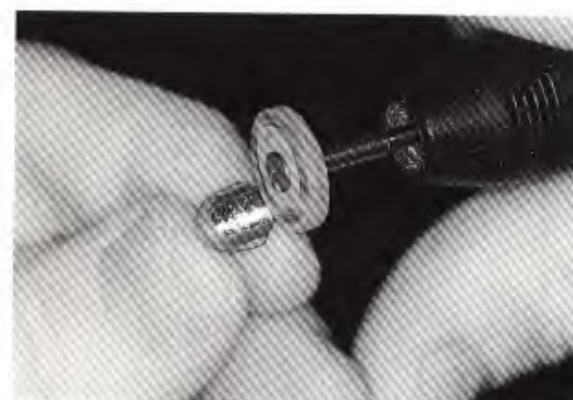
Fig 7-23 For gross finishing use a heatless stone to go over the facial surface.
