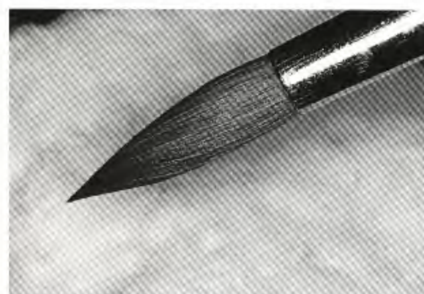
Fig 8-42 The resultant brush should have a distinct sharp "point." Alternatively, many technicians prefer to wet their brush by placing it in their mouth and simply twisting it. Although the technique may be different and less hygienic, the result is virtually the same and the loose-bristled brush is "pointed."
