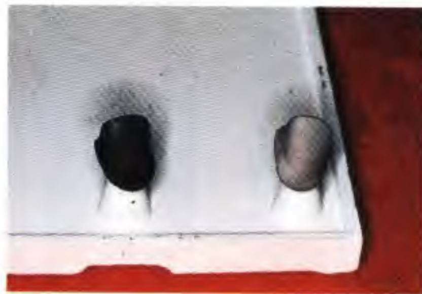
Fig 6-10 The difference in appearance of the oxidized castings is even more distinct when comparing the same high palladium-copper unit ( left ) to a coping made from a palladium-silver (tin only) alloy ( right ). Note that the palladium-silver alloy produces a relatively thin layer of a light gray oxide.
