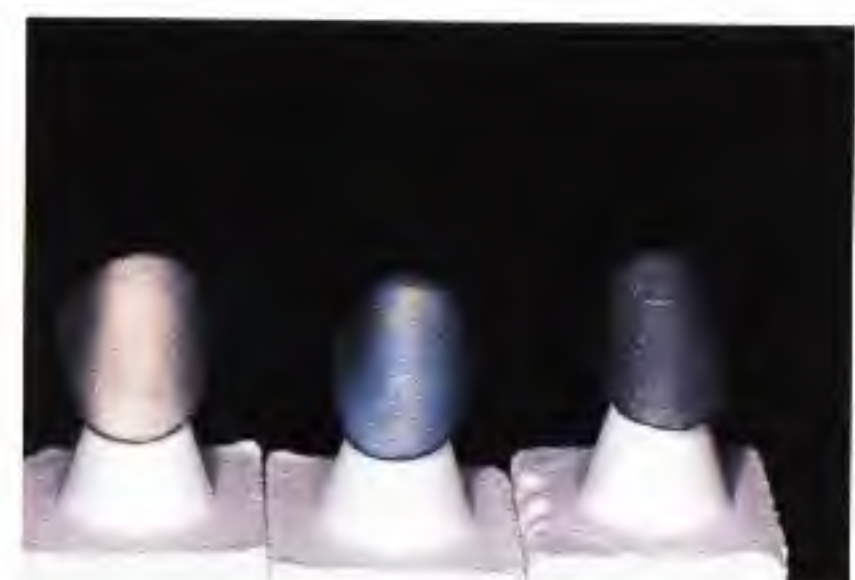
Fig 6-11 These are three different types of base metal alloy (Ni-Cr-Be, left ; Ni-Cr beryllium free, middle ; and Co-Cr, right ). They each form a distinctive colored oxide layer when oxidized.
