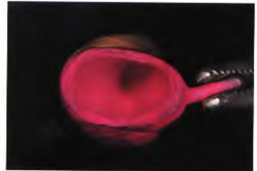
Fig 7-12b A casting after being sprayed with Occlude has a thin, uniform layer of the disclosing medium.
