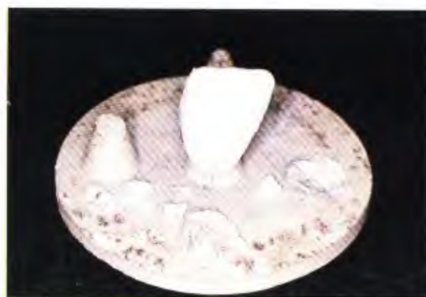
Fig 8-74 This wet porcelain buildup was either not dried long enough or was suddenly exposed to high heat so that the moisture in the porcelain produced steam, which caused portions of the buildup to "pop off" the metal substructure.
