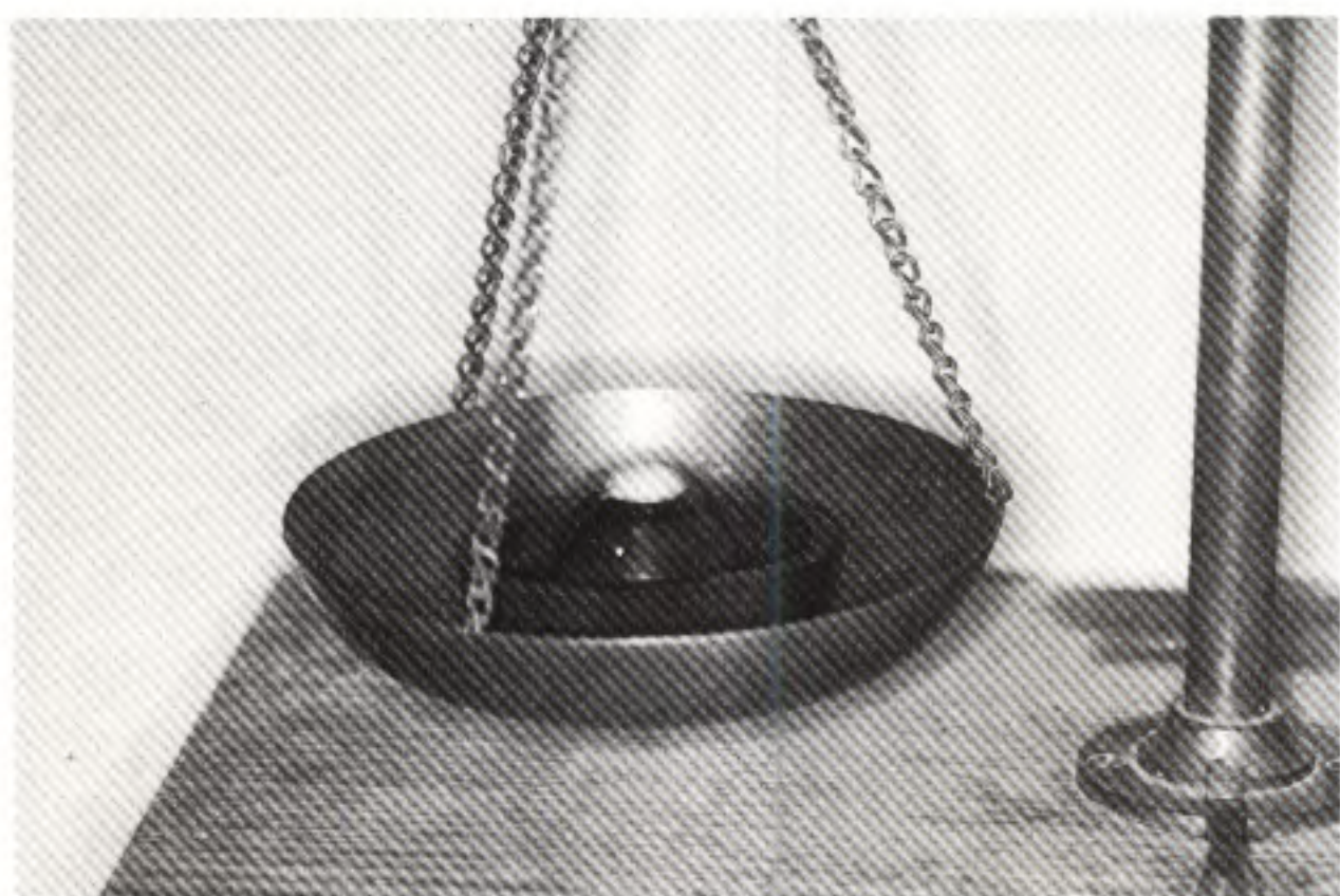
Fig 5-11 The opening in the crucible former is filled with wax and the orientation dot is placed. The crucible former is placed on a scale and weighed. The weight of the crucible former can be permanently recorded on the base with an indelible pen.
