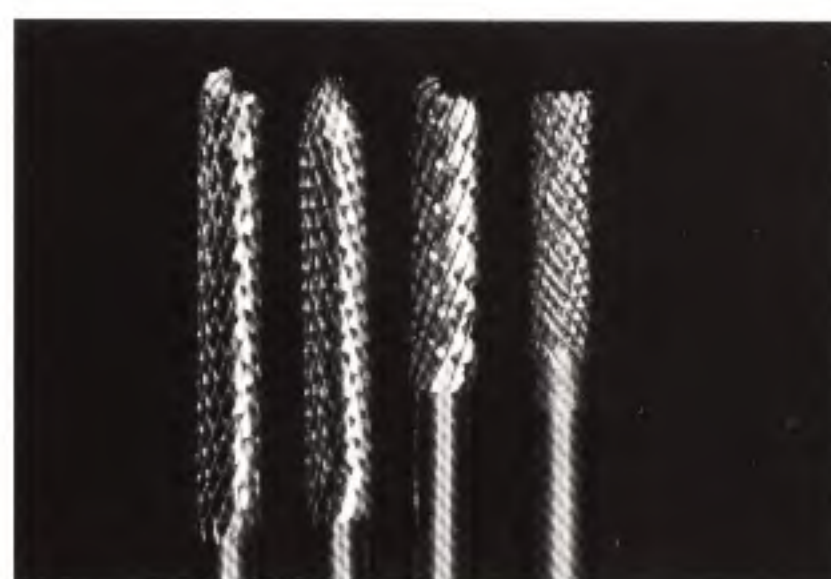
Fig 7-7 Assorted carbide burs for adjusting and finishing the porcelain-bearing areas of a metal substructure (Brasseler USA, Inc). Note the varied shapes and designs.
