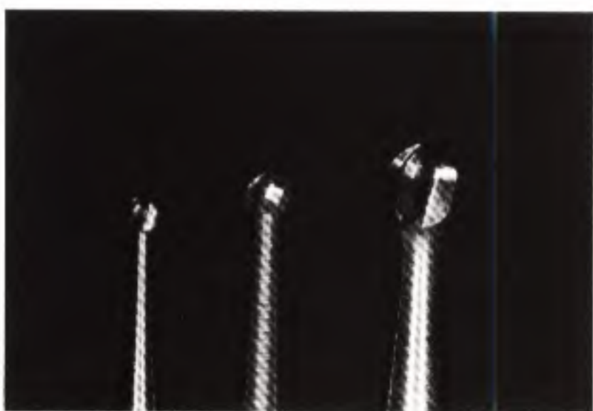
Fig 7-6 Assorted round carbide burs: no. 1/2 ( left ), no. 2 ( middle ), and no. 8 ( right ) used for fitting and adjusting.
