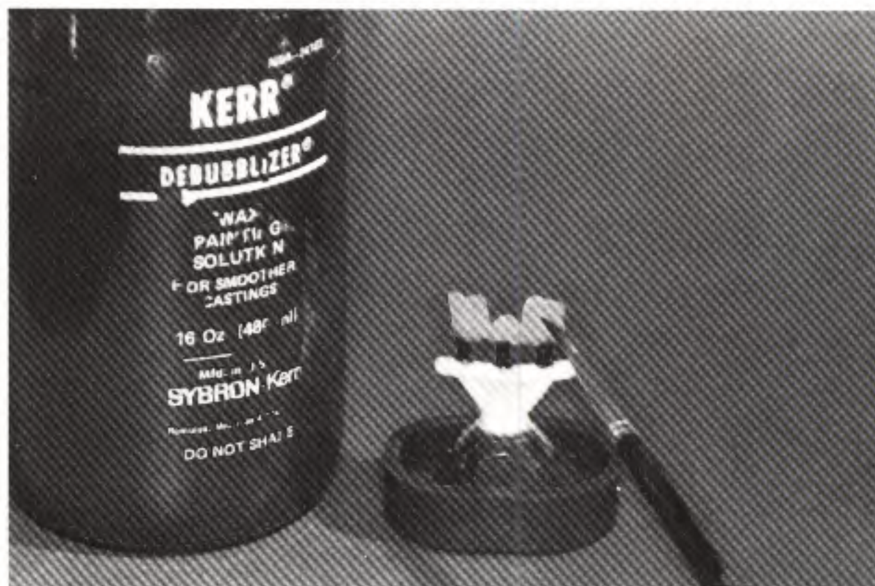
Figs 5-29a and b Apply a thin layer of debubbler (wax pattern cleaner) to the wax patterns and indirect spruing system and allow it to dry thoroughly before investing. Then weigh the assembly again and determine the amount of alloy needed (see Appendix C).
