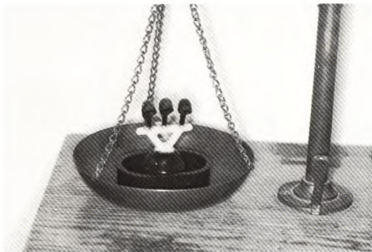
Fig 5-12 A prefabricated wax sprue former, with attached wax patterns, is placed in the crucible former, and the entire assembly is weighed.
