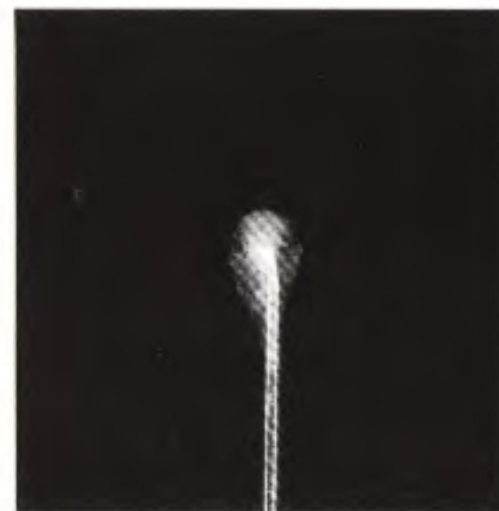
Fig 7-58 Insert one end of the solder strip in a properly adjusted torch until the end rounds. The rounded end of the solder strip after heating.
