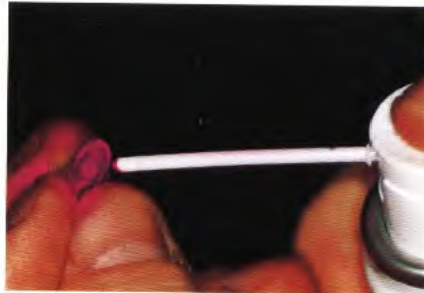
Fig 7-12a Occlude (Pascal) sprayed into the inside of a casting.
