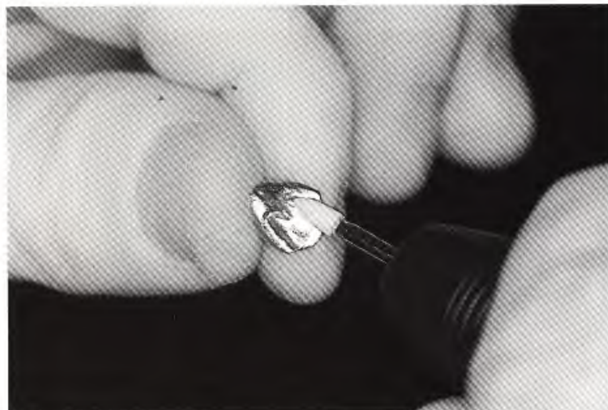
Fig 7-33 If the lingual surface is rough or contains irregularities, use a brown stone. Otherwise, a smooth casting generally will only require a gentle finishing with a fine white ceramic stone.
