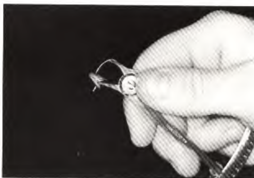
Fig 7-22 The metal calipers should be used to measure the thickness of metal before any adjustments are made (Iwanson gauge, Pfingst Co). Hold the gauge securely and allow the movable area to close on the casting. The thickness of metal will be indicated on the scale at the base of the gauge.
