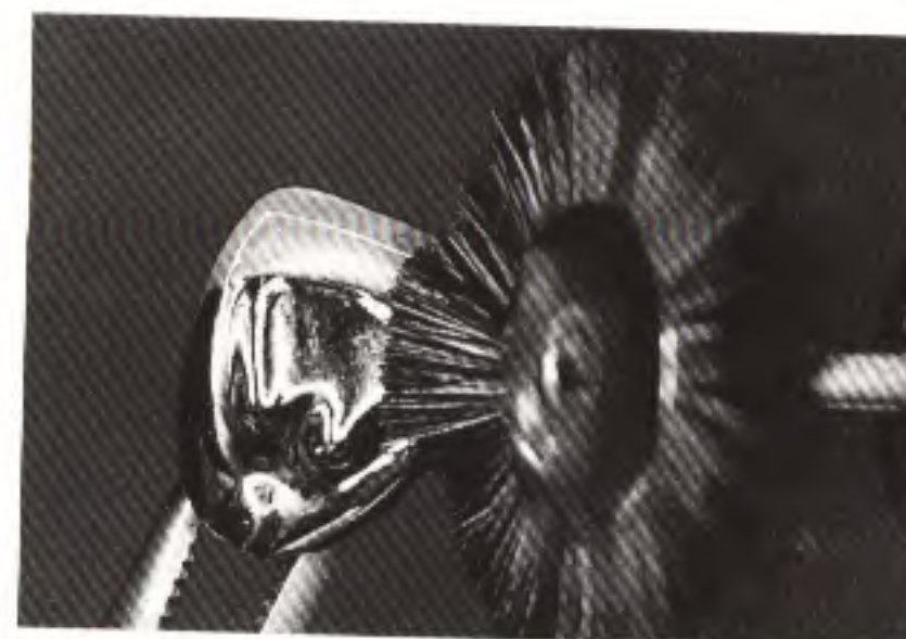
Fig 9-59 Slowly rotate the brush in the BBC abrasive, and the brush will pick up the polishing compound. Using light pressure and great care, slowly rotate the brush loaded with BBC over the metal surface. As the procedure is mentioned previously, try to avoid bringing the polishing compounds in contact with the glazed porcelain. After the metal surface has been polished with BBC, remove all the residual polishing compound with a steam cleaner or ultrasonic cleaner before moving on to a high shine.
