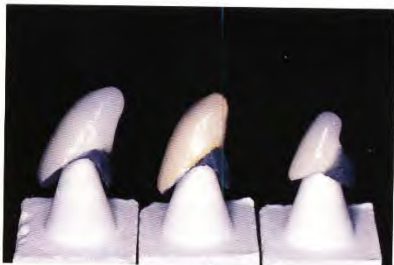
Fig 3-2 Three different brands of dental porcelain were all fired on copings made from the same palladium-silver alloy. However, the two nongreening porcelains ( left and right ) maintained their resistance to discoloration by silver after five body bakes whereas the conventional porcelain ( middle ) discolored substantially after two firings.
