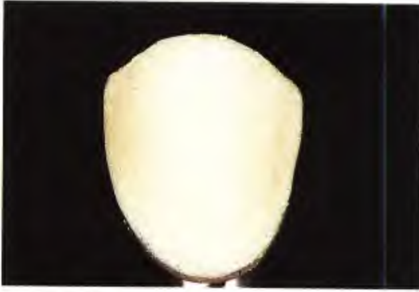
Fig 8-27 A properly fired (sintered) opaque layer should have a sheen or eggshell glisten.
