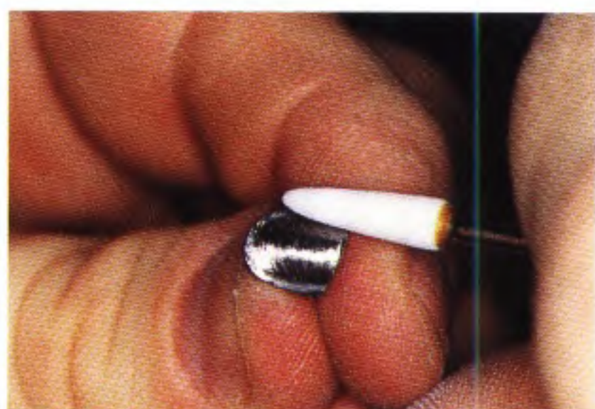
Fig 7-26 With the stone rotating counterclockwise, begin finishing at the porcelain-metal junction opposite you. Move the stone across the metal surface towards you. When you reach the porcelain-metal junction nearest you, stop and repeat the process so the direction of finishing is always toward you.
