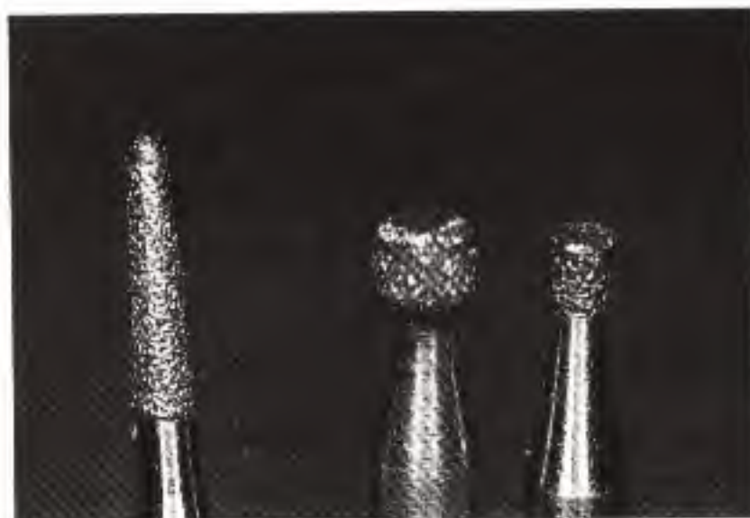
Fig 9-2 Diamond abrasive instruments are available in a variety of shapes, sizes, and grits, making them useful for all phases of adjusting and finishing.
