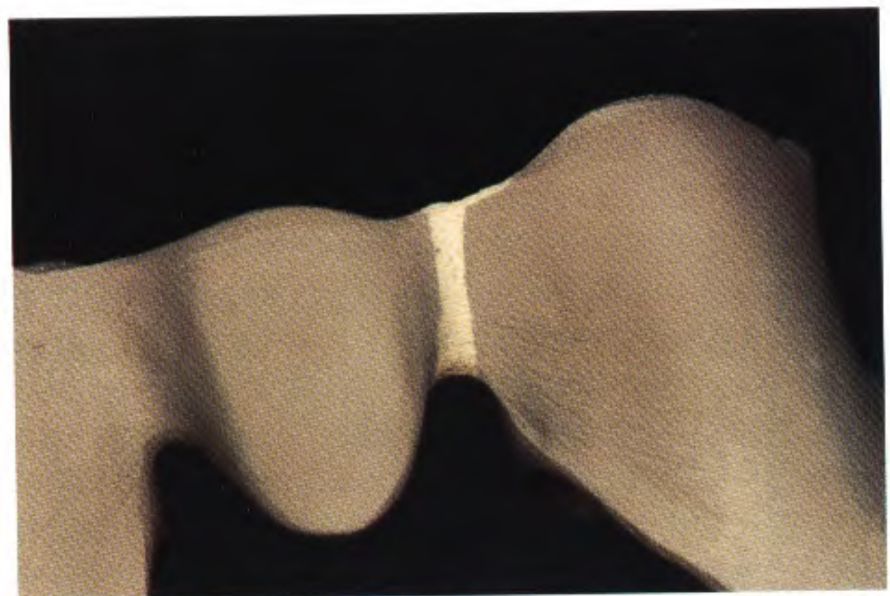
Fig 7-75 Close-up view of the solder joint after oxidation. The yellow hue of the presolder is readily evident, as is the fact that the solder joint is dense and free of contamination and porosity.
