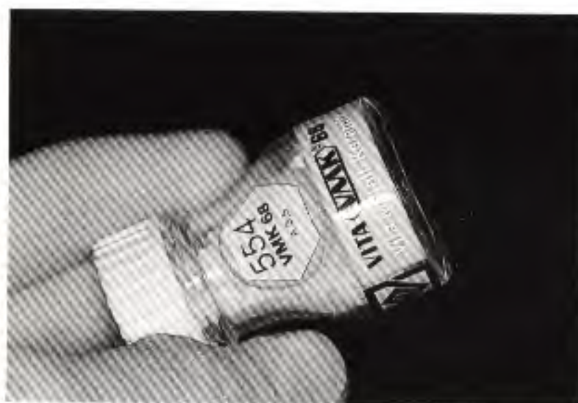
Fig 8-35 Tumble each porcelain jar before dispensing to thoroughly distribute any fine particles that may have settled during storage.
