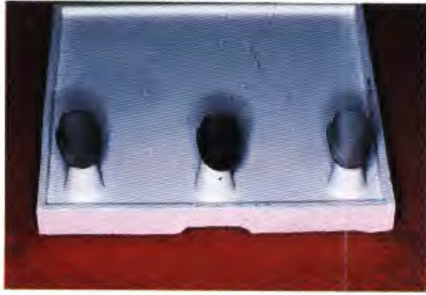
Fig 6-9 All three of these oxidized copings were made with noble alloys, yet their color and character (texture, thickness, etc) differ markedly in appearance. The Olympia casting ( left ) is medium gray and has a moderate level of oxidation. The high palladium-copper alloy ( middle ), Naturelle, has the darkest color (dark brown to black) and the greatest amount of oxidation. The Will-Ceram W-1 casting (a palladium-silver alloy, right ) is light gray and apparently has a thin oxide layer.
