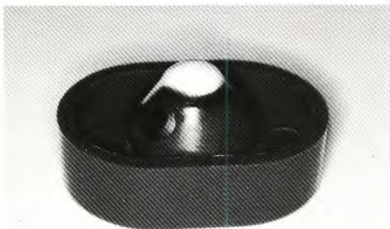
Figs 5-6a and b A wax orientation dot on the crucible former ( left ) will be picked up by the investment ( right ) and help you to locate the trailing edge of the wax patterns for casting.
