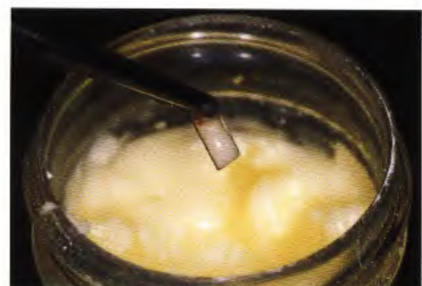
Fig 7-68 A fluoride-containing flux for presoldering (High Fusing Bondal Flux, Williams Dental Co). A properly mixed flux should be moist and have a smooth, creamy consistency. Dip the cut solder strip in the pre-solder flux. Simply wipe off any excess so that only a light coating remains.
