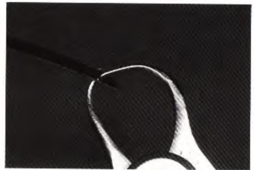
Fig 7-52 Use the metal calipers to measure the thickness of the solder strip (Iwanson gauge, Pfingst Co). This strip of presolder measures 0.3 mm in thickness.
