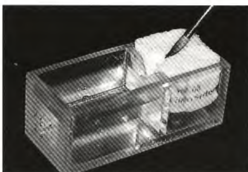
Fig 8-41 Continue rotating the brush as it is dragged out of the distilled water and across the sponge.
