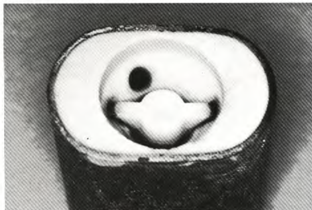
Figs 5-6a and b A wax orientation dot on the crucible former ( left ) will be picked up by the investment ( right ) and help you to locate the trailing edge of the wax patterns for casting.
