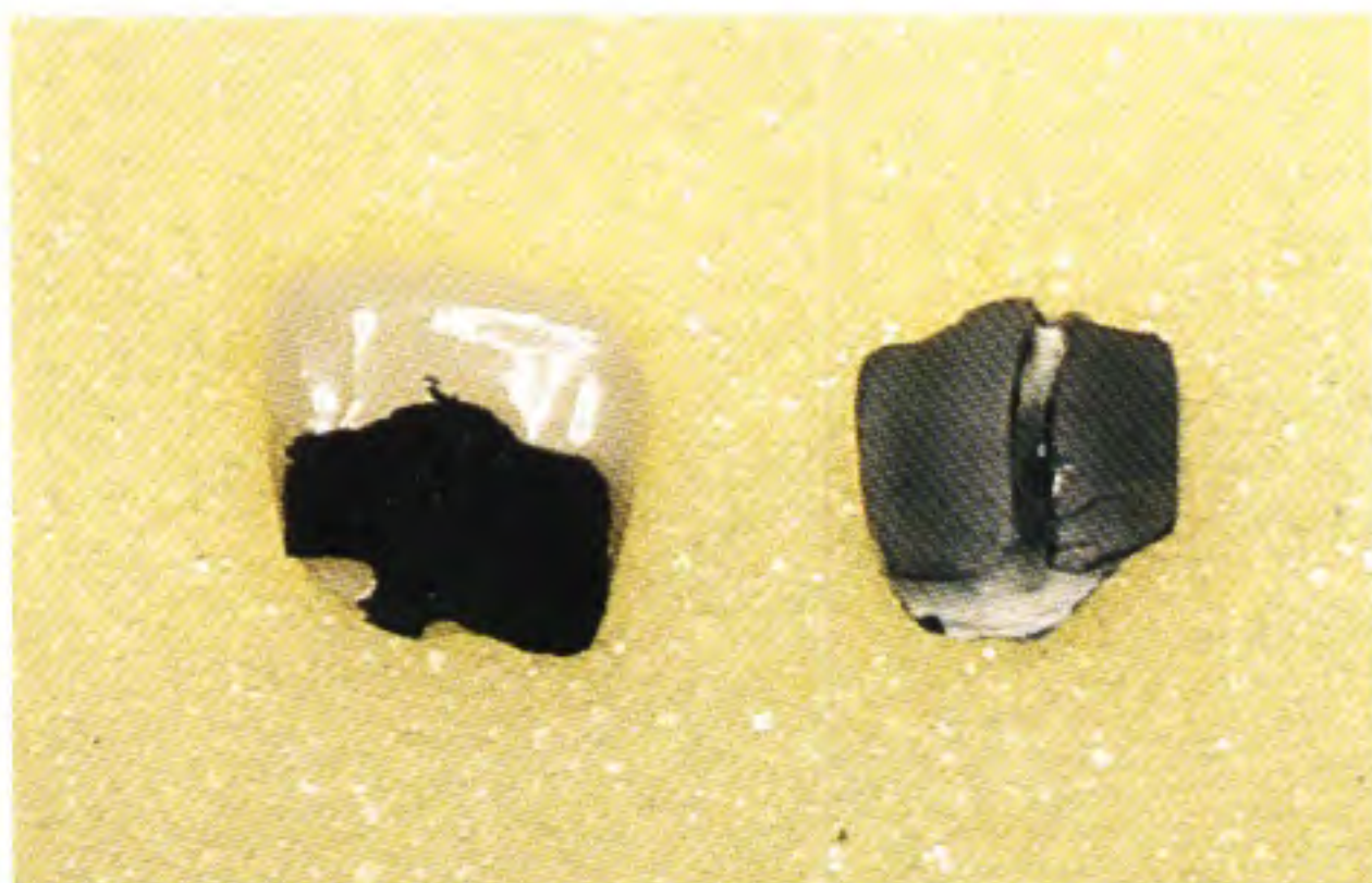
Fig 6-14a Note how the heavy greenish oxides bonded to the porcelain ( left ) yet a substantial amount of oxidation remains on the metal substructure ( right ) of this cobalt-chromium casting.
