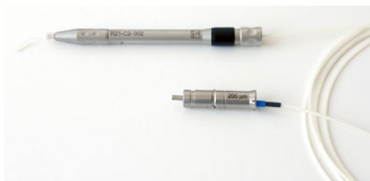
Fig. 4.11 Hallow handpiece for thin optic fibers (200–300 μm) that permits the passage of the fiber up to the extremity (typically for the near-infrared laser)
