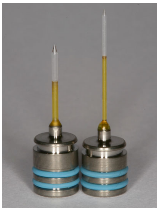
Fig. 11.19 PIPS™ tips: 9 mm long, 600 μm diameter tip (left) and 12 mm long, 400 μm diameter tip (right)
