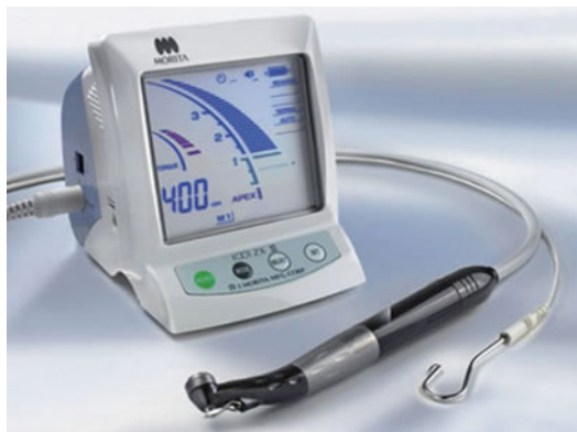
Fig. 11.96 Electronic apex locator (Root ZX by Morita) used to confirm anatomical length
