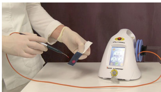
Fig. 5.5 The fiber/tip activation is performed at 1 W on dark-blue articulating paper, repeating the procedure 4–5 times up to seeing the tip becomes darker
