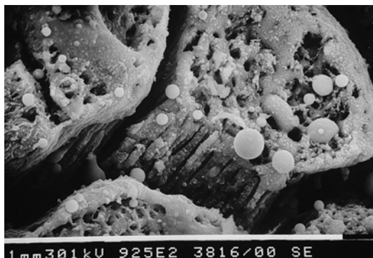
Fig. 6.4 SEM image of radicular dentin irradiated with Nd:YAG laser at 1.5 W, 100 mJ, 300 \mu s pulse duration, with a 200 micron fiber (2 mm/s speed). Bubbles of recrystallization and cracks resulted from laser thermal damage (Imagine courtesy of Prof. V. Kaitsas Rome (Italy))
