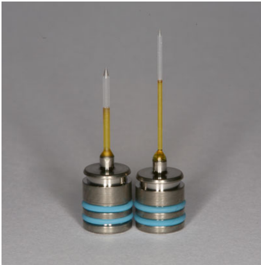
Fig. 5.12 Radial and stripped PIPS tips of 400 and 600 \mu\text{m} diameter, 14 and 9 mm long, respectively, for Er:YAG laser (LighWalker, Fotona; Slovenia)
