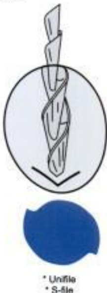
Fig. 8.17: Cross section and longitudinal shape of S-file
