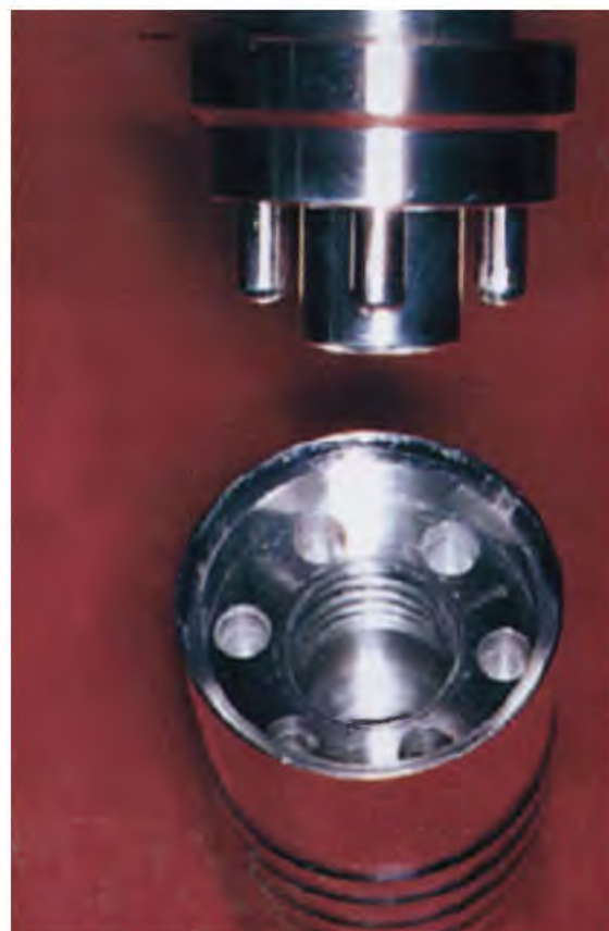
FIGURE 22-11. Park Dental Research has designed an internal antirotational modification. The abutment has protruding extensions, which slide into female components in the top of the implant.
