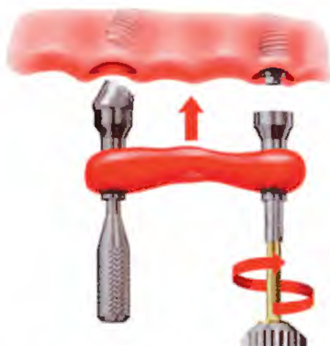
FIGURE 18-19. The anterior abutments are used as a positioning reference for the jig, which is needed to attach the 30-degree rotational abutments to the posterior implants. (Courtesy Nobel Biocare, Yorba Linda, Calif.)
