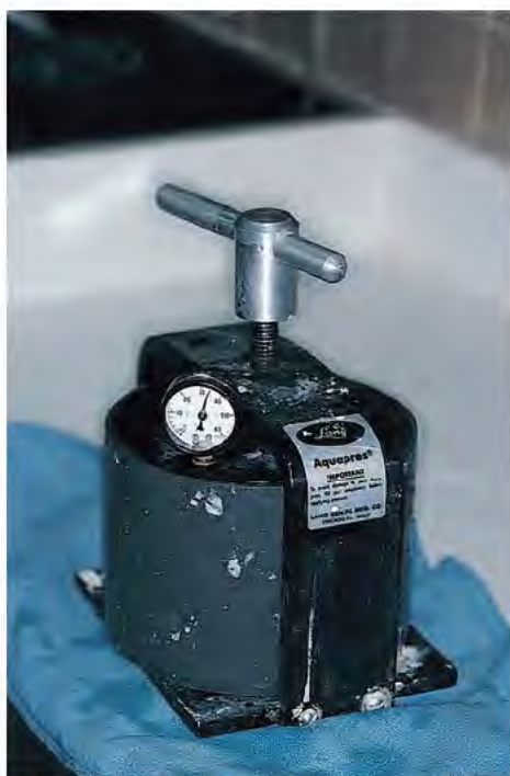
FIGURE 20-4. The pressure pot is filled with hot water, and the Lang duplicator is placed in it at 30 psi for 30 minutes to allow the acrylic to set completely.
