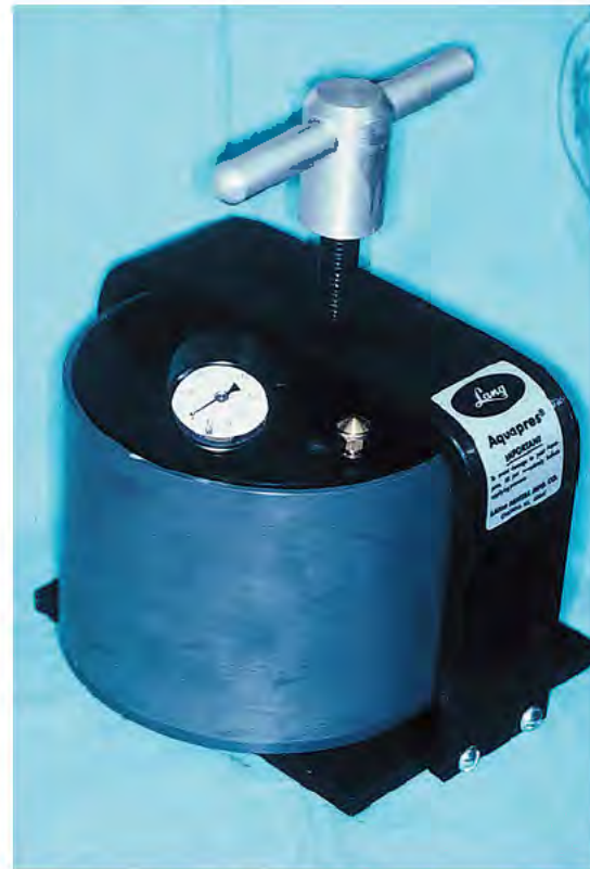
FIGURE 4-30. In the curing of acrylic denture replicates, the pressure pot is filled with hot water to the point of overfilling and then closed tightly; this allows the acrylic to cure fully and without bubbles.
