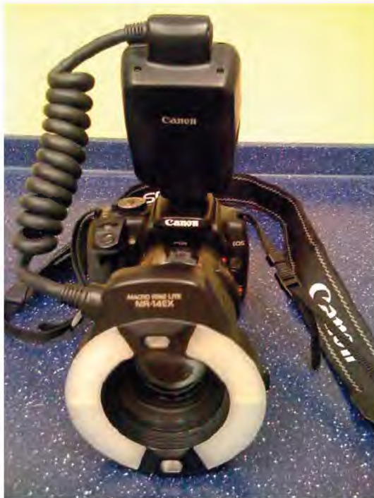
FIGURE 4-58. A Digital SLR camera with synchronized external ring flash and a macro zoom lens.
