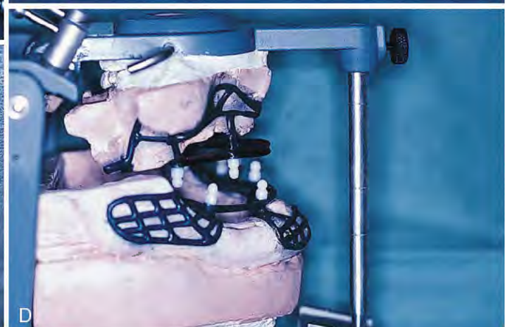
FIGURE 14-32. A , Positive, screw-free retention can be achieved by surveying a stereolithographic cast and marking the points of widest dimension. B , An infrastructure should extend slightly into undercut zones. Screw holes are included for elective use. C , The wax-up with bar and O-ring attachments, when cast, will move into place only if tapped with a mallet and orangewood stick. It then fits quite firmly. D , Waxed implants must be related to each other or to the opposing denture so that occlusal forces are directed optimally through their infrastructures. For the CT scan method, these relationships are achieved only by using the tube and stylus technique.
