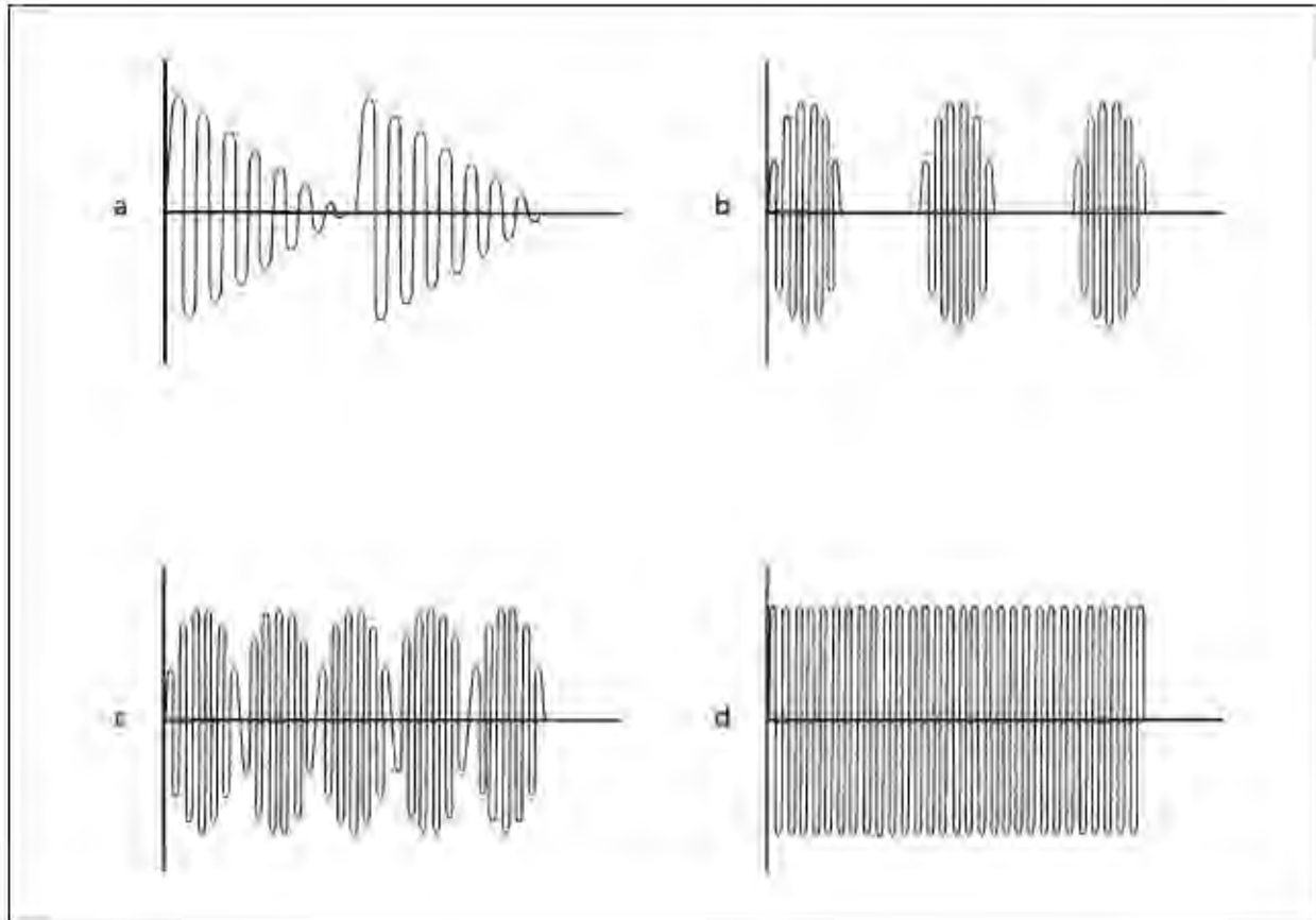
Fig 16-30 Four forms of electrosurgery current: (a) unrectified, damped; (b) partially rectified, damped (half-wave modulated); (c) fully rectified (full-wave modulated); and (d) fully rectified, filtered (filtered).
