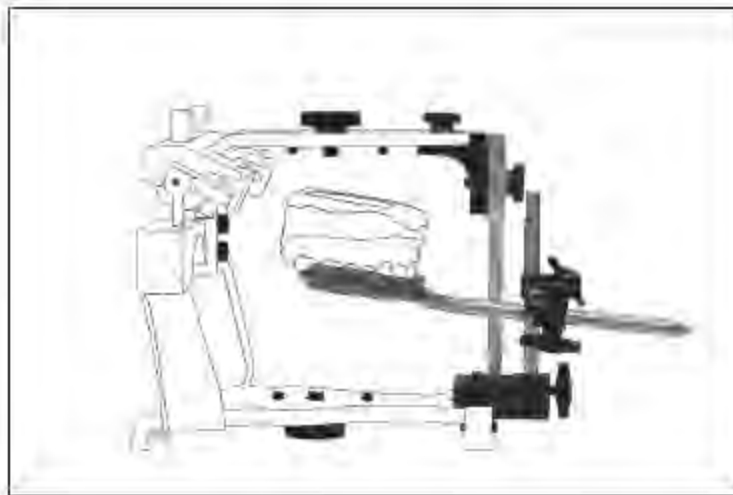
Fig 5-47 The maxillary cast in the bite fork is positioned by the articulator index.
