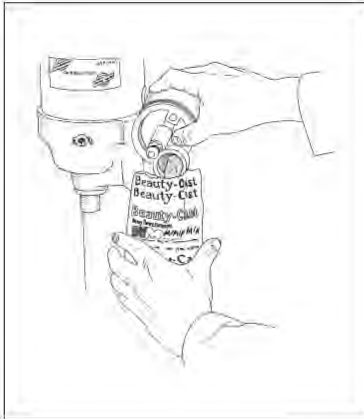
Fig 20-10 Unused investment is vibrated into the original envelope and disposed of in a trash receptacle.
