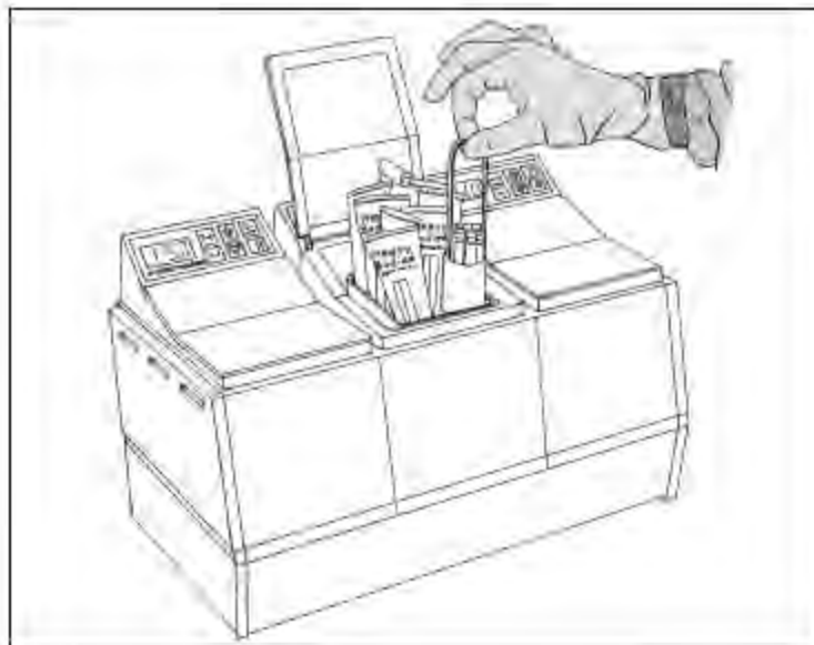
Fig 17-9 A cartridge of liquefied hydrocolloid is removed from the storage bath.
