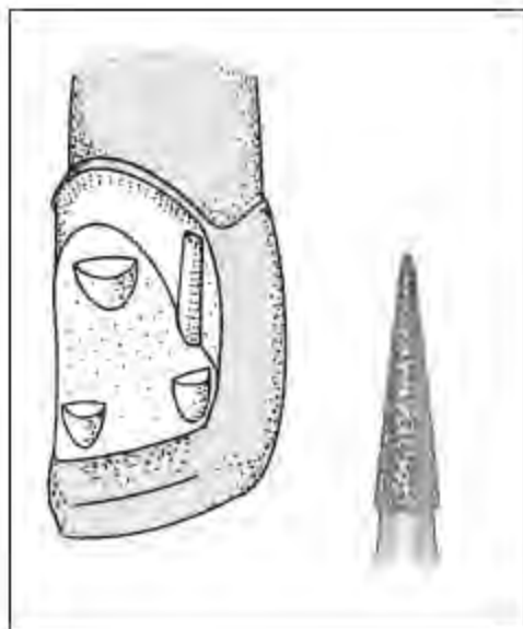
Fig 11-58 Lingual axial reduction: round-end tapered diamond.
