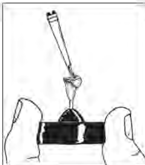
Fig 20-22 It may be necessary to paint phosphate-bonded investment into the wax pattern with a small brush.
