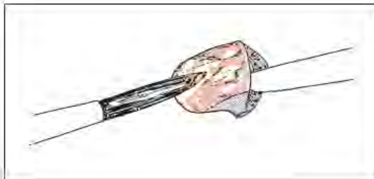
Fig 24-26 A thin “wash layer” of opaque porcelain is applied with a brush.
