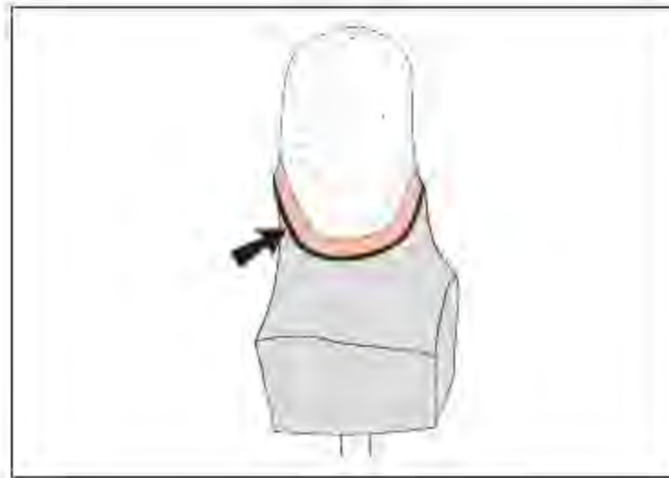
Fig 24-39 Following the first firing of the shoulder porcelain, porcelain shrinkage will cause a slight marginal gap (arrow).
