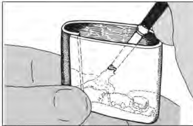
Fig 26-14 Investment is brushed into the retainers.
