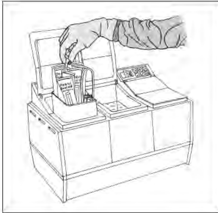
Fig 17-4 Tubes and cartridges of hydrocolloid are placed into the liquefying bath.
