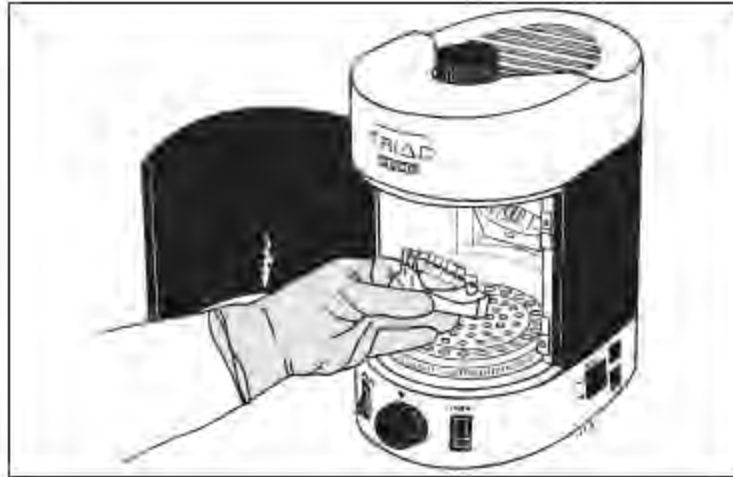
Fig 15-46 The cast with the resin-loaded template is placed in the light-polymerizing unit.
