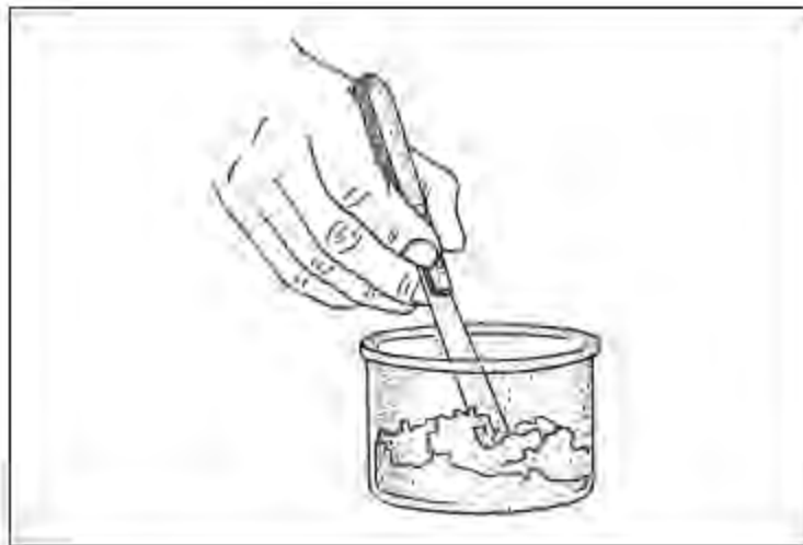
Fig 20-7 Investment is wetted completely by hand spatulation.
