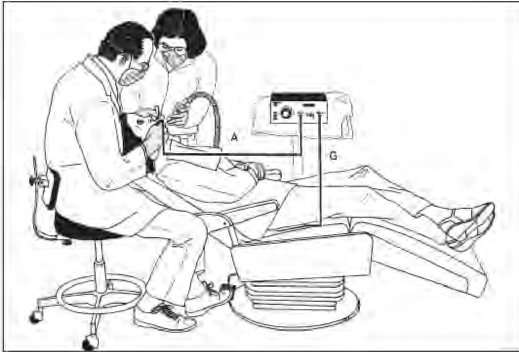
Fig 16-31 Electrosurgical current flows from the unit to the active (cutting) electrode (A) to the ground (G) and back to the unit.
