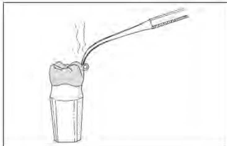
Fig 21-9 The ring is luted to the wax pattern.
