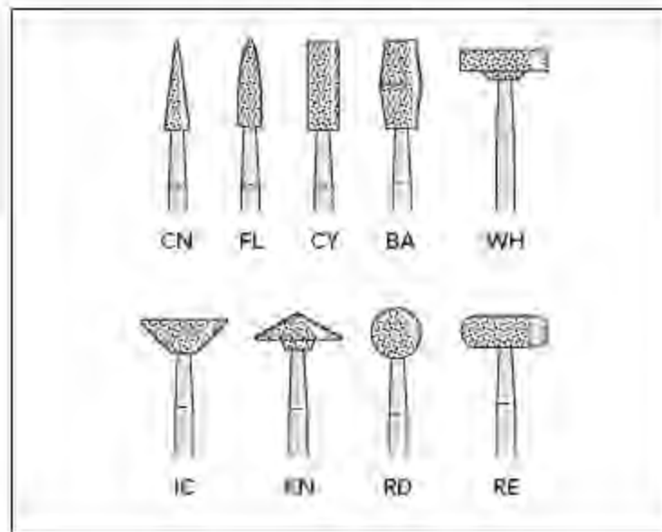
Fig 21-2 Common shapes of abrasive stones are: cone (CN), flame (FL), cylinder (CY), barrel (BA), wheel (WH), inverted cone (IC), knife edge (KN), round (RD), and round edge (RE).
